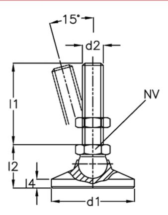
A/F = 12 d1 = 25 d2 = 8 l1 = 50 l2 = l4 = -Static load (N) = 7 Weight in (g) = 57
